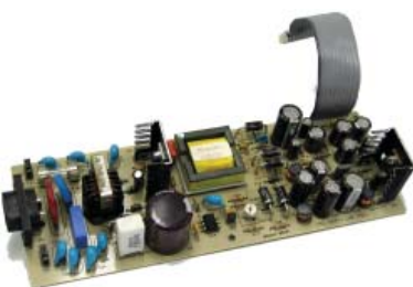
Part-SMPS/UEC Switch Mode Power Supply Suit UEC-660
